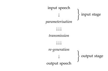
Fig. 1. A vocoder. The multiple arrows indicate that the parameterised representation of speech typically has several distinct groups of parameters – e.g., filter coefficients capturing the spectral envelope and source parameters such as the fundamental frequency F0.
