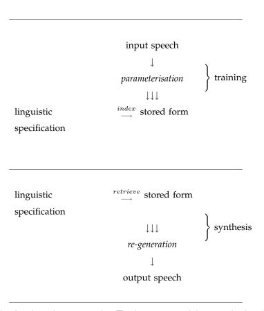
Fig. 2. Speech synthesis, viewed as a vocoder. The input stage of the vocoder has become "training" and is performed just once for the entire speech corpus (training data). The output stage of the vocoder has become "synthesis", which is performed once for each novel sentence to be synthesised.
