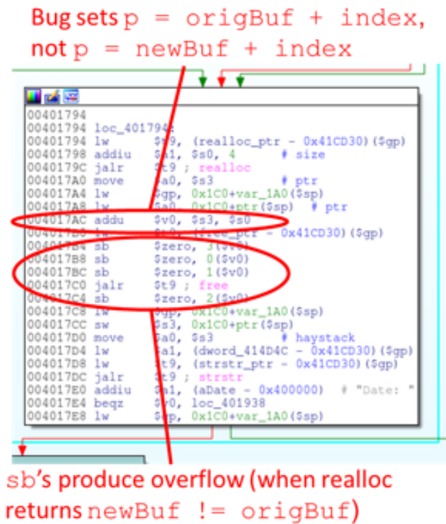
Fig. 6. A real ARE-discovered buffer-overflow flaw where the programmer uses the old pointer value rather than the potentially new pointer value from realloc
