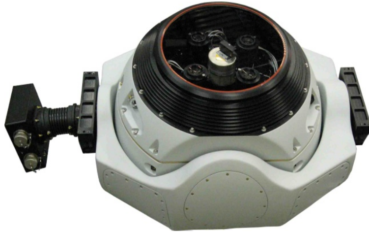
ARGUS-IS system components. Left: sensor in 25" gimbal; Right: CFPA with 92 5 MPixel FPAs.
