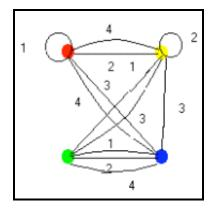
To solve the puzzle, you need to find in this combined graph two separate subgraphs that each use all four nodes just once and each of four edges, numbered from 1 to 4. Moreover, each node would have only two edges (or the two ends of a loop) emanating from it. One subgraph would represent the four front-back pairings, and the other would represent the four top-bottom configurations.
