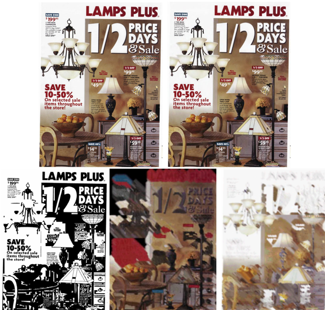
Figure 2. Example catalog page. Top left: compressed with JPEG (650 kbytes) and SLIm (107 k). Bottom: SLIm components; left to right: Mask (43 k), Foreground (34 k), and background (29 k)
