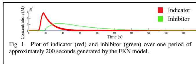
Fig. 1. Plot of indicator (red) and inhibitor (green) over one period of approximately 200 seconds generated by the FKN model.
