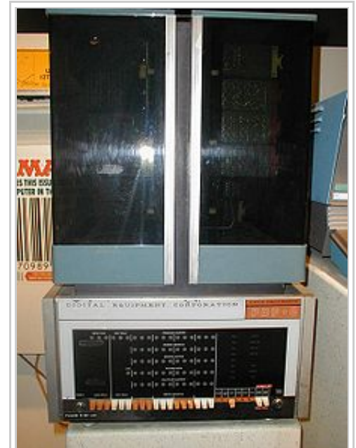
A PDP-8 on display at the Smithsonian's National Museum of American History in Washington, D.C.. This example is from the first generation of PDP-8s, built with discrete transistors and later known as the Straight 8 .
